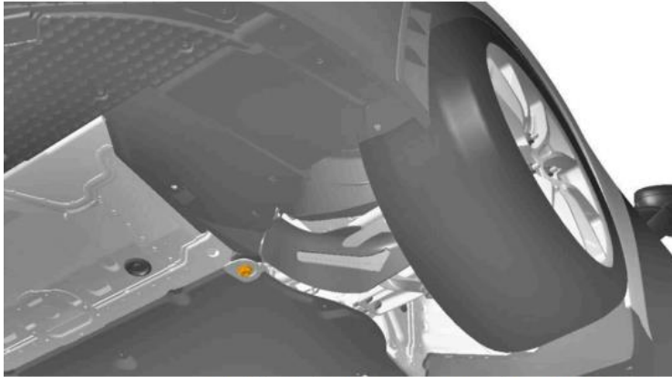
Fig. 22: Height measurement (base), front axle
